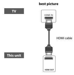
When connecting with an HDMI cable, the audio signal will be output as the digital audio signal simultaneously, so you do not need the analog audio connection described on page 6.
